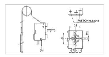
Electrical contact capacity = NC 16(6) / A 250 Vac Switches = changeover Max. head temperature = 85°C Min. capillary curvature radius = 5 mm Connection = via faston 6,3x0,8 Certifications = CE, ENECO3, EAC, UL
